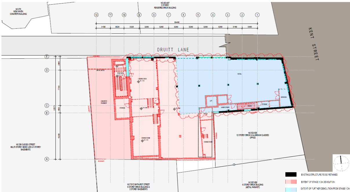
Figure 7: Proposed indicative demolition plan - basement 1
