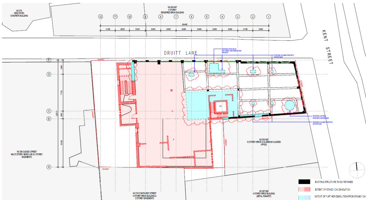
Figure 10: Proposed indicative demolition plan - level 2
