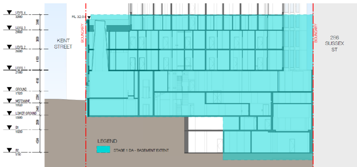
Figure 21: Comparison of the approved basement extent and that of the Detailed Design DA
